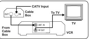
With this connection you can view/record any cable channel including scrambled channels to which you have subscribed.
